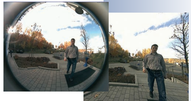
Image section with correction of wide-angle distortion
