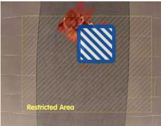
**"Restricted Area":** With camera firmware version MX-V4.4.0.31 or higher an event can also be triggered if something enters a "digitally marked," rectangular restricted area within the image. Up to 20 different restricted areas can be activated simultaneously for each camera by creating multiple profiles. Active restricted areas can be hidden or made visible within the image by selecting the desired color and transparency.
