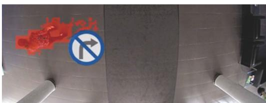
**"Turn":** Using the behavioral detection it is possible to detect whether an object is leaving the path defined as main direction. An event is triggered when an object deviates in an angle larger than 45° and smaller than 135° from the defined main direction axis (here: from the virtual line between 12 and 6 o'clock).
