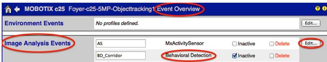
Click on the button **Edit...** To configure such a new profile, you can select one of the "alarm types" (Corridor, Duration of Stay ...) and set other parameters as required.
