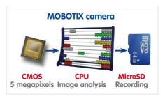
record video. This means that you do not have to rely on expensive, overloaded video management software as most of the important functions that require a large amount of processing power are integrated into the MOBOTIX cameras themselves.
