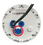
Remove bayonet catch and USB plug: Turn the bayonet catch to the left (red arrow in figure), take it off and remove the blue USB plug.
