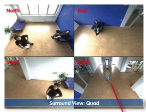
Each of the four views features a software-controlled pan/tilt/zoom function (virtual PTZ), allowing it to be customized as necessary.
