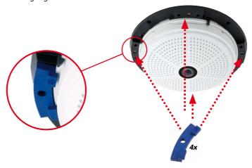
Mount the stainless steel cover: Position the stainless steel cover as shown and tighten the security screws using the included two-hole driver bit.
