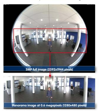
**Example**: The people marked by the red circle in the middle area of the image would not have been recorded by a regular PTZ camera; the full image recording of the Q25M allows to determine for example, the exact time at which the people entered the image area recorded by the camera. A **Browser** (Internet Explorer with MxPEG ActiveX plug-in), **MxControlCenter** or **MxEasy** can be used to examine the recorded sequences.
