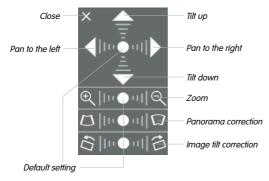
To use the OnScreen Control, click on the arrows in the top area for shifting the image section. In the bottom areas, which are displayed when needed, click to the left and/or right of the center point.
