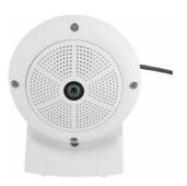
The Stand/Wall Mount is a useful accessory for testing and for finding the optimum mounting position of the camera. The set also includes an Allen wrench as well as a Torx screw with dowel and the corresponding Torx wrench for installing as alternative wall mount for testing.
