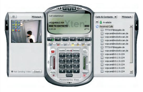
The requirements and the configuration for SIP video telephony are mostly identical to those of SIP voice telephony (see section 9.2, *VoIP Settings for IP Telephony*). The only difference is the **Video** parameter in **Admin Menu > VoIP Settings**, which has to be set to *Enabled*.
