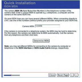
Enter a unique MSN that is still available for your telephone number. Make sure that this MSN is not identical with that of any other device on this ISDN bus. This means that you can operate e.g. a telephone, a computer and a MOBOTIX camera simultaneously on the same ISDN bus.
