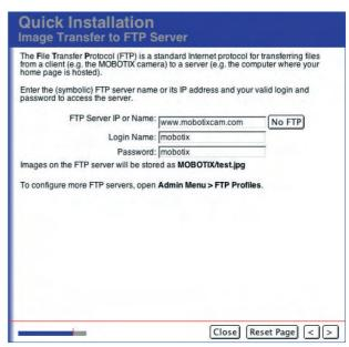
your domain has been set up. In the **FTP Server IP or Name** field, you can enter either the domain name (e.g. www.mobotix.de) or a (numeric) IP address. In any case, make sure to enter the correct user name and password for the FTP connection.
