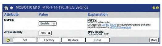
If the camera would output an uncompressed color image with  $640 \times 480$  pixels (e.g. as a bitmap image), the file created (and thus each individual live image) would be about 1 MB in size. Transferring this file to the user's computer using an ISDN connection would take about 2 minutes or using a 10 Mbps Ethernet connection still 1 second. It is easy to see why this format is not suitable for transferring and storing image data at high frame rates.
