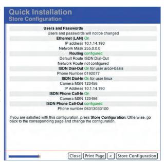
Please note that the new network settings will be in effect after rebooting. If you have changed the camera's IP address, you can access the camera using this new IP address after rebooting. The original factory default IP address (see sticker on the camera case) will no longer be valid.
