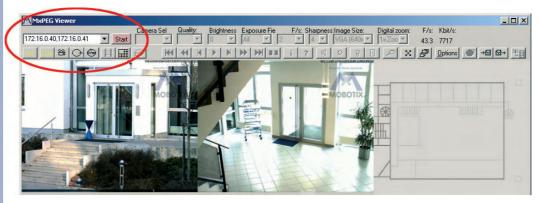
MxViewer displays the live images of the cameras it has found; the values for frame rate and bandwidth in the top right corner show the combined values for all displayed cameras. Clicking on a camera will activate this camera (yellow frame) and the frame rate and bandwidth values will be those of the active camera.
