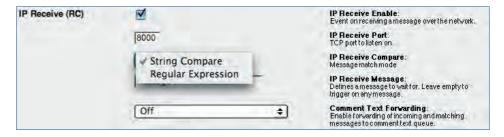
To trigger an alarm using network messages: **RC**
