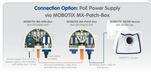
This connection option uses the Ethernet installation cable instead of the patch cable to establish the data connection and PoE power supply. This is helpful, if e.g. an IP camera on a high pole is connected to the network installation cable via the MOBOTIX MX-Patch-Box and the power and network connections are to be supplied through the installation cable at the bottom of the pole using the MX-NPA-Box.
