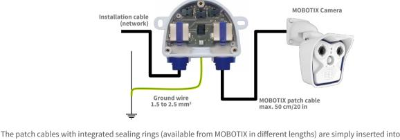
the RJ45 connectors and fastened using the bayonet catch (1 patch cable to end device, 1 patch cable to PoE switch/injector). The ground wire is attached at the center (only qualified electricians are allowed to do this!).
