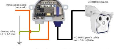
This variant allows using a network installation cable to the PoE switch. The wires are inserted into the LSA terminal in the center, while the MOBOTIX patch cable connects to the camera. The ground wire is attached at the left (only qualified electricians are allowed to do this!).
