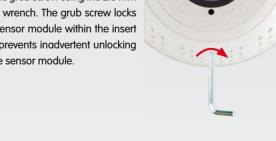
• Adjust the sensor module temporarily by pointing it into the desired viewing direction.
