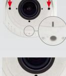
driver to lift the sensor module out of the insert as shown. Take care not to damage the sealing of the sensor module housing.
