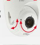
• Make sure that the TOP/OBEN label on the insert is pointing upwards. If this is not the case, loosen the two fastening screws using the 2.5 mm Allen wrench and rotate the insert. Lightly tighten the two fastening screws.
