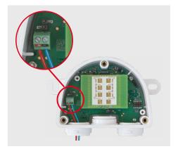
It is highly recommended to test the detection area before installing by covering the front of the MX-Proximity-Box with the material you want to use!
