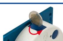
When replacing the SD card, make sure that recording has been deactivated in the browser (**Admin Menu > Storage > Storage on External File Server / Flash Device**; activate recording again in the same dialog).
