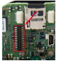
Use one finger to carefully press the board of the module onto the receptacle. Make sure that the MxIOBoard-IC is fully inserted.
