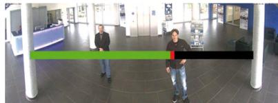
Carefully turn the lens using the red lens wrench in clockwise or counter-clockwise direction until the red area of the focusing aid in the camera image is as small as possible.
