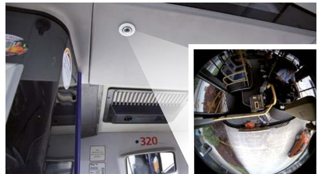
and temperature variations. The ability to exchange the sensor module has proven to be cost-effective and practical, without having to dismantle the whole camera during transportation all recordings are maintained.
