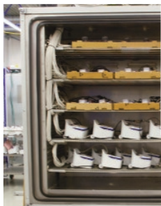
Each camera is tested at extreme temperatures before shipping
