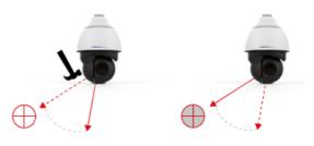
vandalism or environmental vibrations) suddenly exert an influence. The EIS technology can effectively generate stable images by actively recording the targeted motion of the images and compensating for this accordingly; this is particularly helpful when a high zoom level is set and the camera is installed in a place at which the environmental movements (such as from strong wind or trucks driving past) are not always constant.
