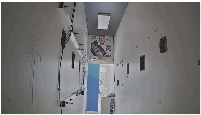
Original MOBOTIX MOVE camera image with activated WDR function: Details are easily recognizable within the dark testing room as well as at the open door with bright light entering through it. The camera automatically combines two differently lit individual images taken within a minimal time difference, thereby forming a live complete image.
