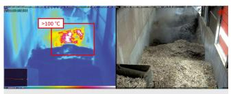
Thermal Radiometry (TR) automatically generates an alarm if the temperature exceeds or falls below the pre-defined temperature range.
