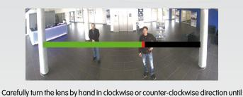
the red area of the focusing aid is as small as possible. Once the focus is adjusted properly, deactivate the focusing aid again (Focusing
