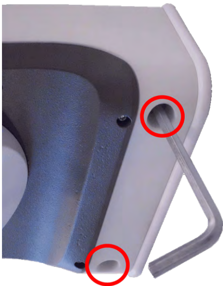
Fig. 30: Tighten Allen screws
