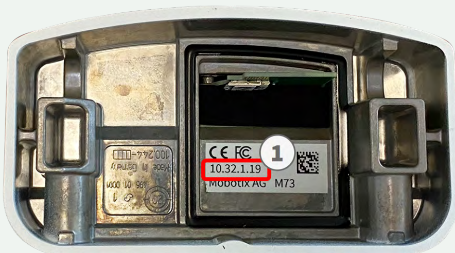
Fig. 5: IP address on the back of the camera housing
