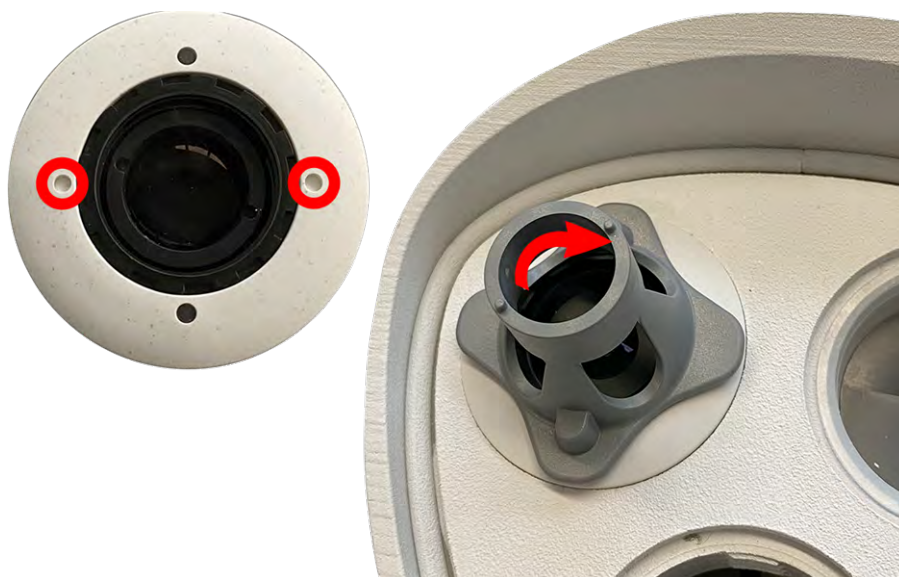
Fig. 11: Lock the sensor module
