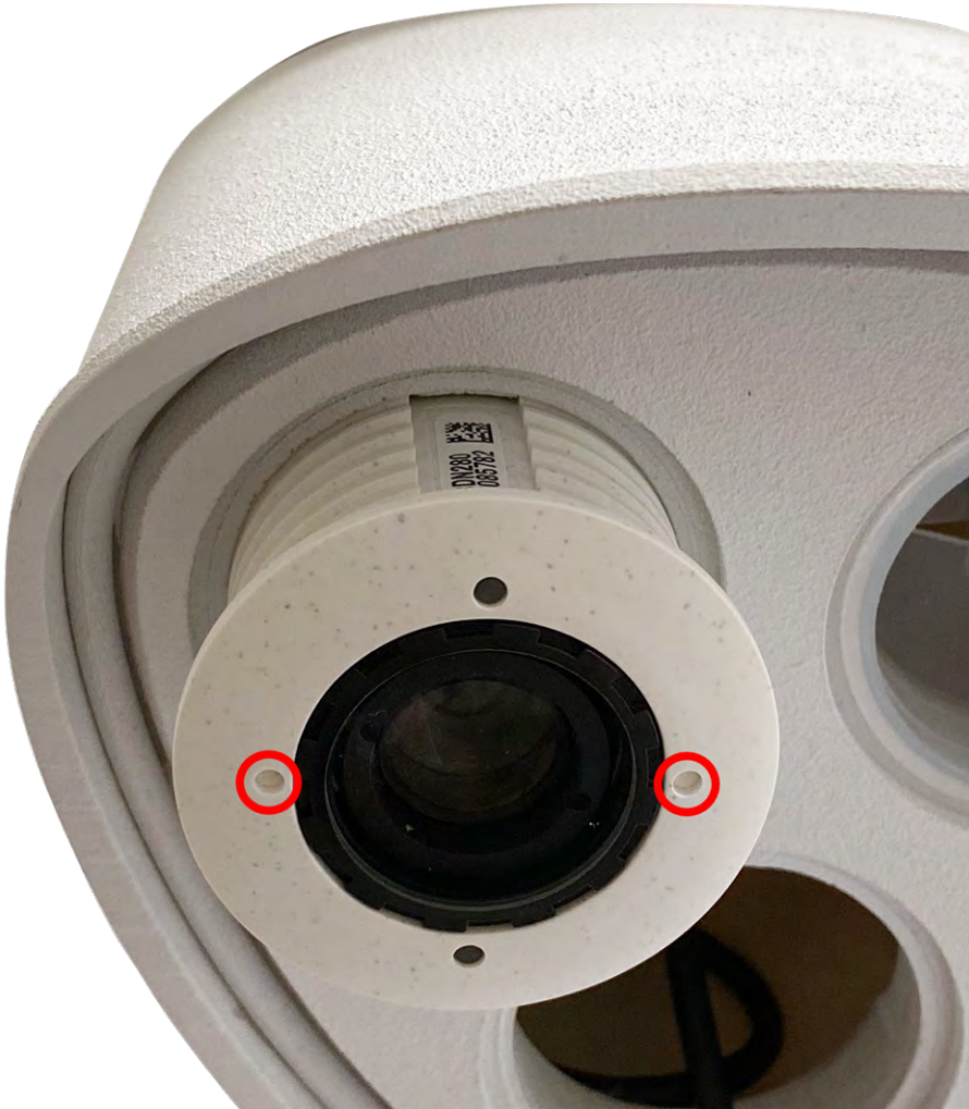
Fig. 10: Insert sensor module into module housing
