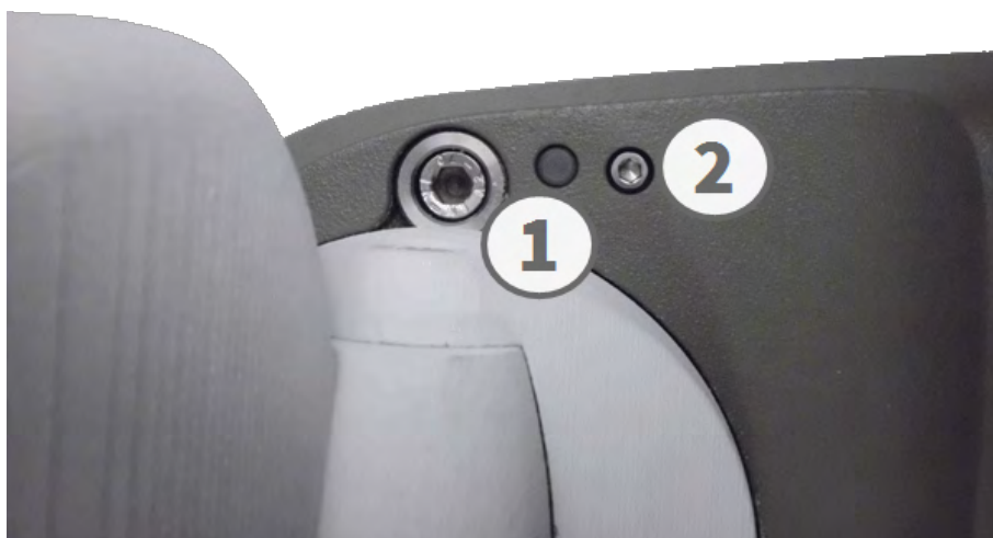
Fig. 34: View of the M73 from below with LED (1) and screw with sealing (2) that hides the key inside the camera body
