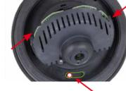
screws (see below) and rotate the main board support to get to these screws. Insert the screws with washers and tighten them.
