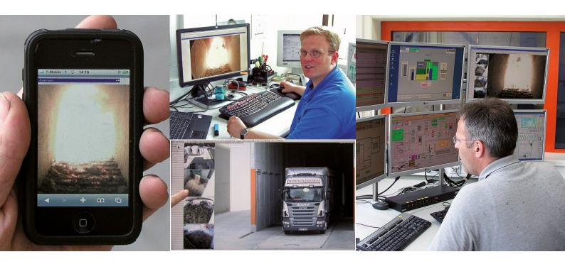
the lens is blown clean again with a compressed air nozzle. And this camera, protected by a dust-proof housing, plays the part perfectly. Another camera on top of the chimney monitors the color and the quanity of the smoke produced. On clear days, it stares directly into the sun for hours without generating burning effects or forming streaks. Cameras with CCD sensors don't have what it takes to stand up to these harsh conditions.
