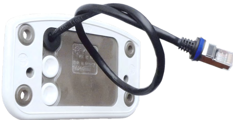
Abb. 33: Network connection of the M73
