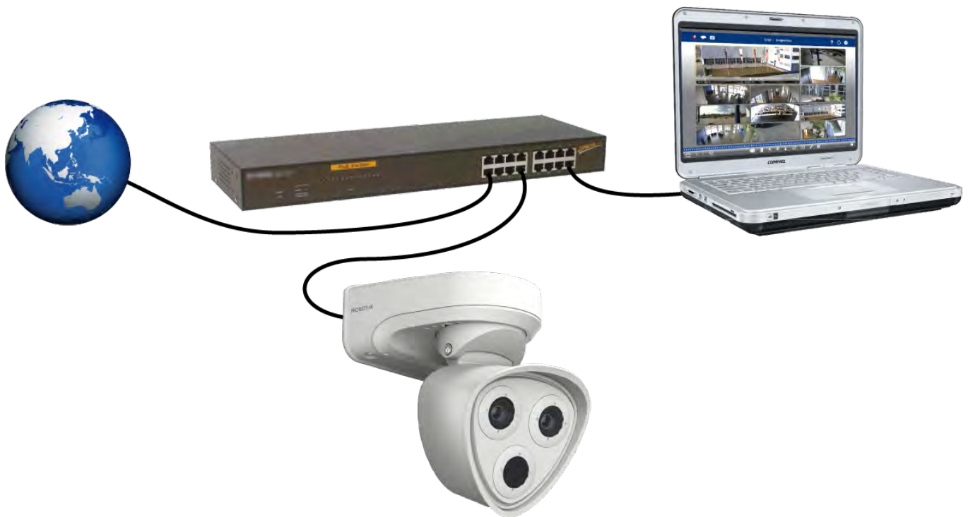
Abb. 36: Power supply using PoE switch according to PoE Plus (802.3at-2009)
