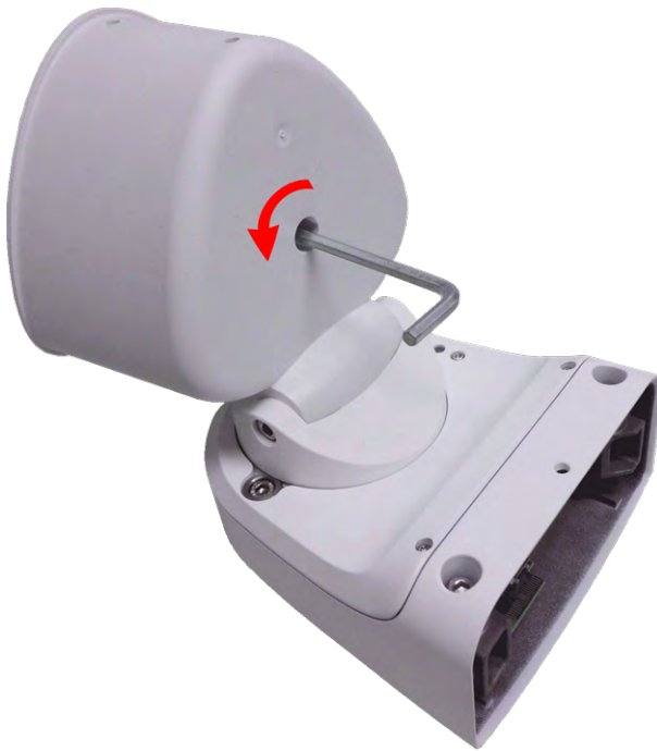
Abb. 12: Opening the Module Housing
