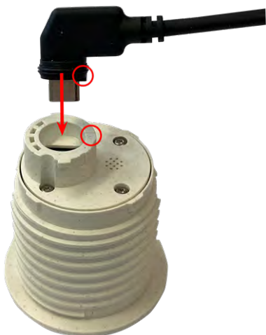
Abb. 27: Connect the sensor module cable
