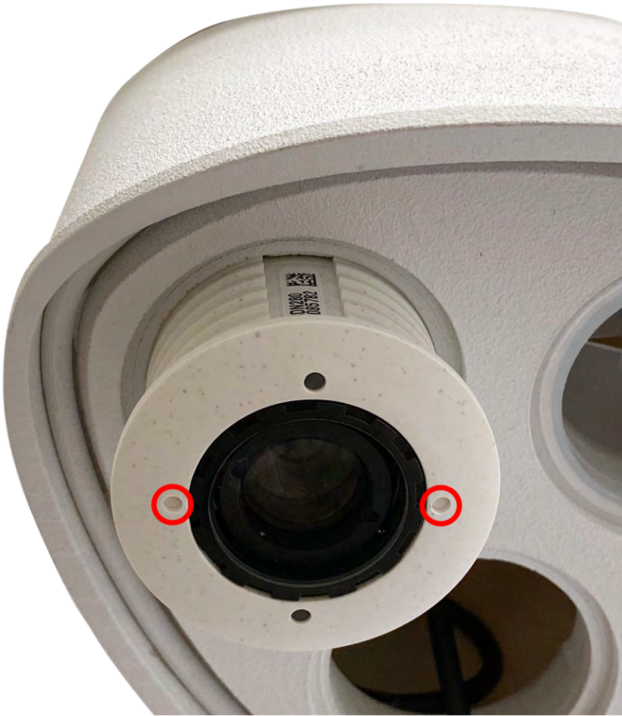
Abb. 24: Remove sensor module from the module housing
