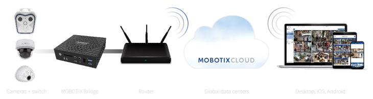
In addition to the MOBOTIX Bridge hardware component, MOBOTIX CLOUD includes video recording, storage and archiving technology, as well as live remote access to any camera, notifications, user management and Internet security — all in one monthly subscription.
