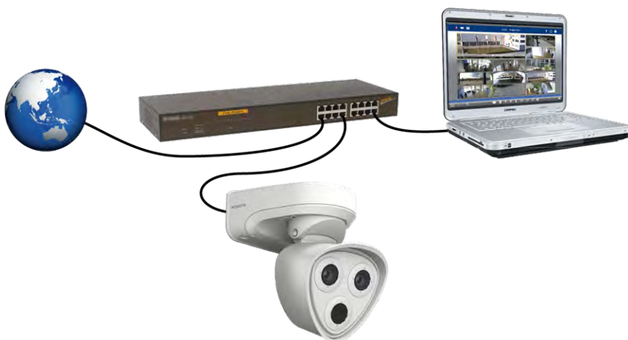
Fig. 35: Power supply using PoE switch according to PoE Plus (802.3at-2009)
