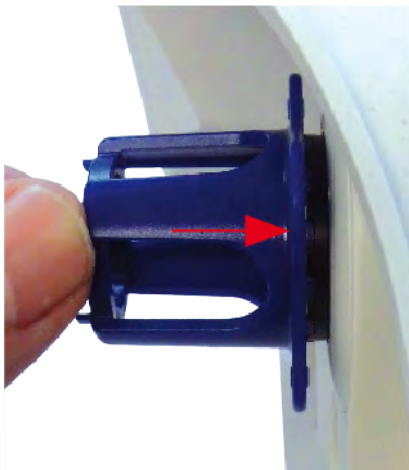
Fig. 58: Push hard to insert lens protection glass and turn to lock
