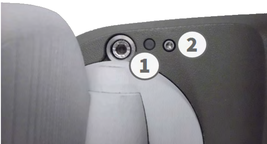
Fig. 46: View of the M73 from below with LED (1) and screw with sealing (2) that hides the key inside the camera body
