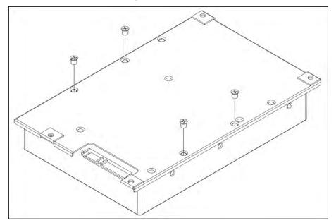
4. Mount the HDD rack back to its original position. No SATA cable required; the HDD is connected auto-
