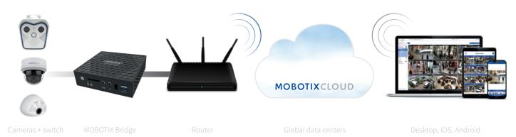
In addition to the MOBOTIX Bridge hardware component, MOBOTIX CLOUD includes video recording, storage and archiving technology, as well as live remote access to any camera, notifications, user management and Internet security — all in one monthly subscription.
