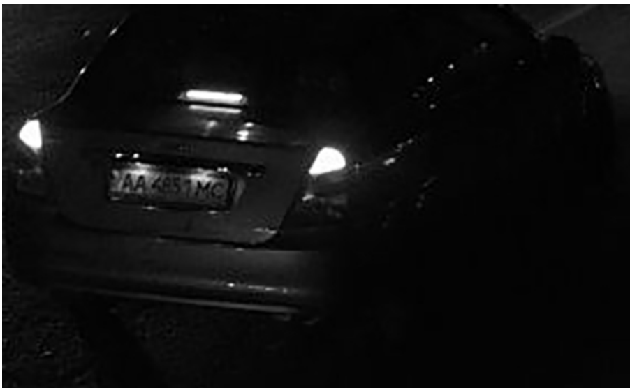
Fig. 15: Insufficient light to recognize license plate
