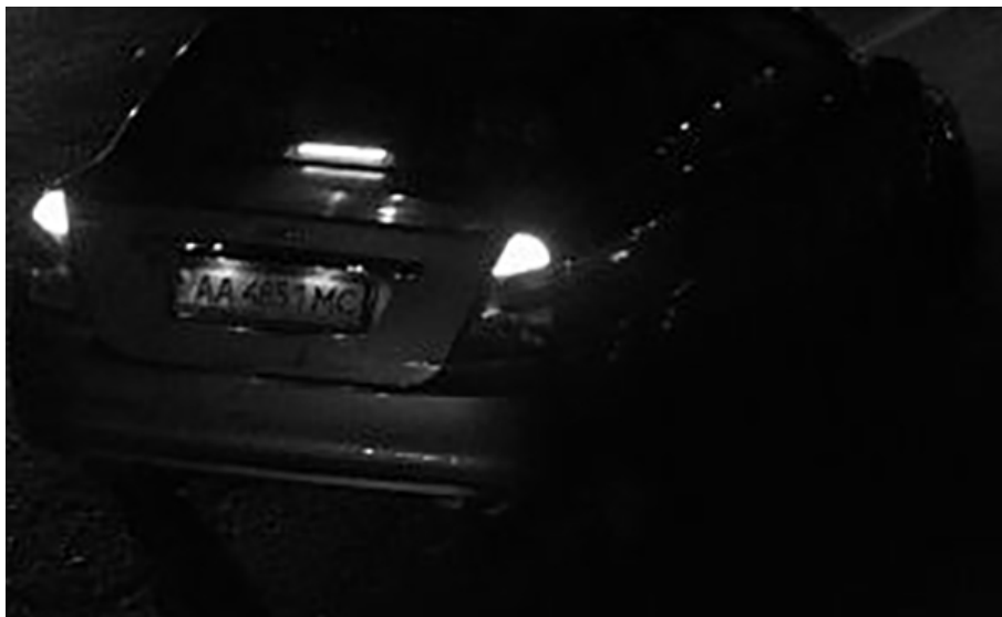
Fig. 15: Insufficient light to recognize license plate
