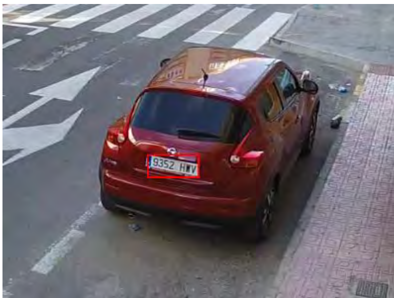
Fig. 16: Insufficient light to recognize license plate
