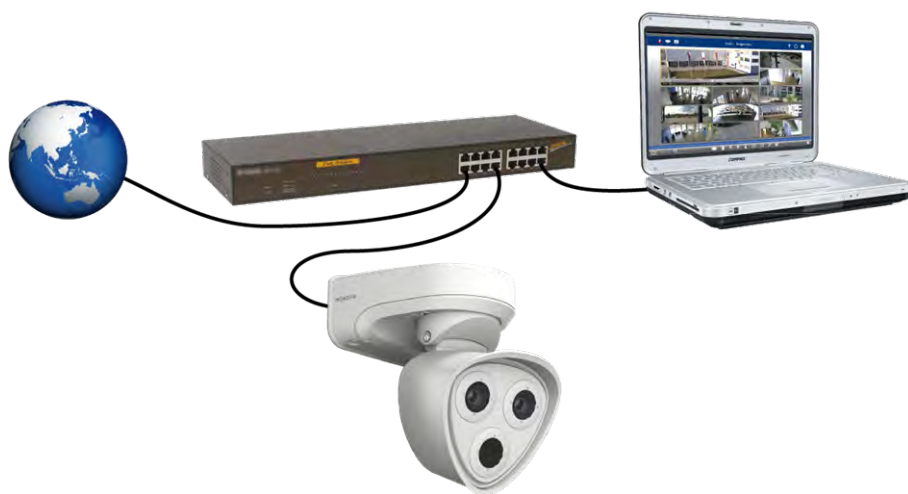
Fig. 54: Power supply using PoE switch according to PoE Plus (802.3at-2009)
