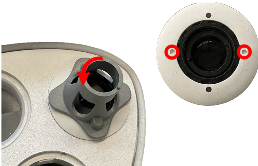
Fig. 24: Unlock the sensor module
