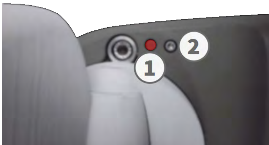
Fig. 76: View of the M73 from below with LED (1) and screw with sealing (2) that hides the key inside the camera body
