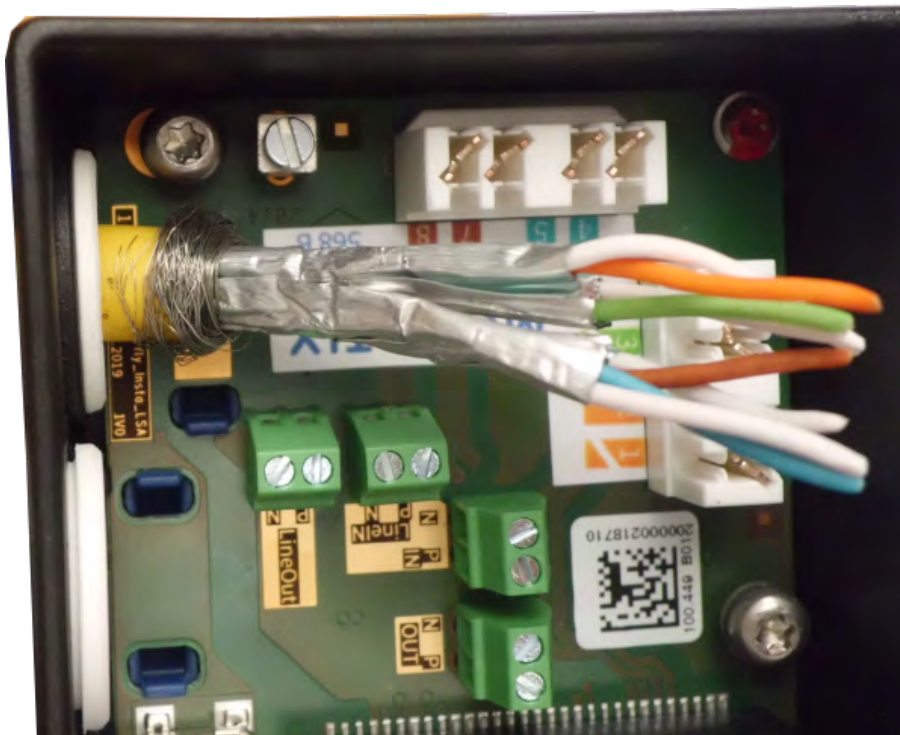
Fig. 62: Network cable inserted, plug properly seated
