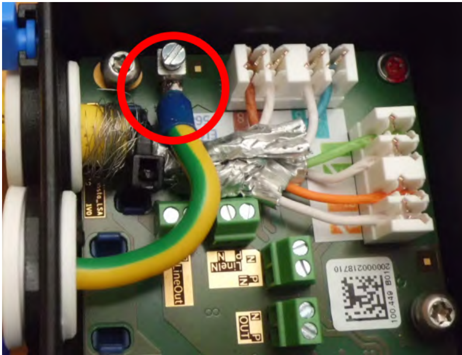
Fig. 68: Ground wire connected to terminal
