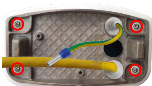
Fig. 60: Mounting plate with ground wire and network cable
