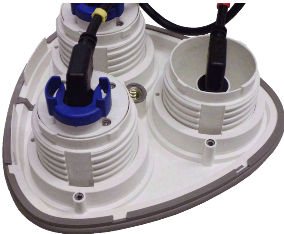
Fig. 15: Default front plate with sensor modules (back)
