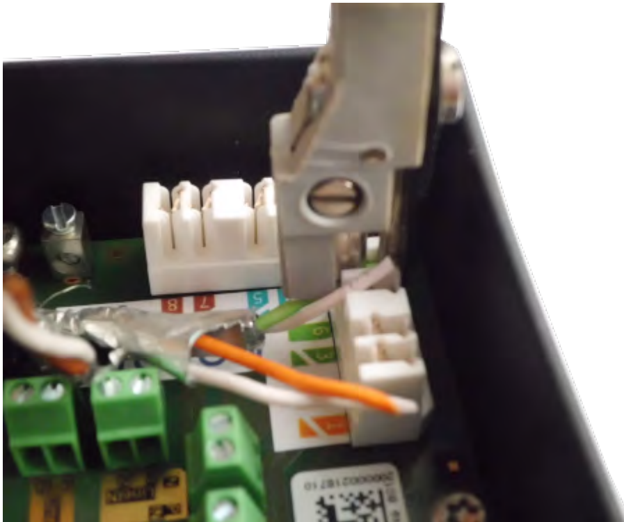
Fig. 65: Network wires connected using LSA+/Krone tool
