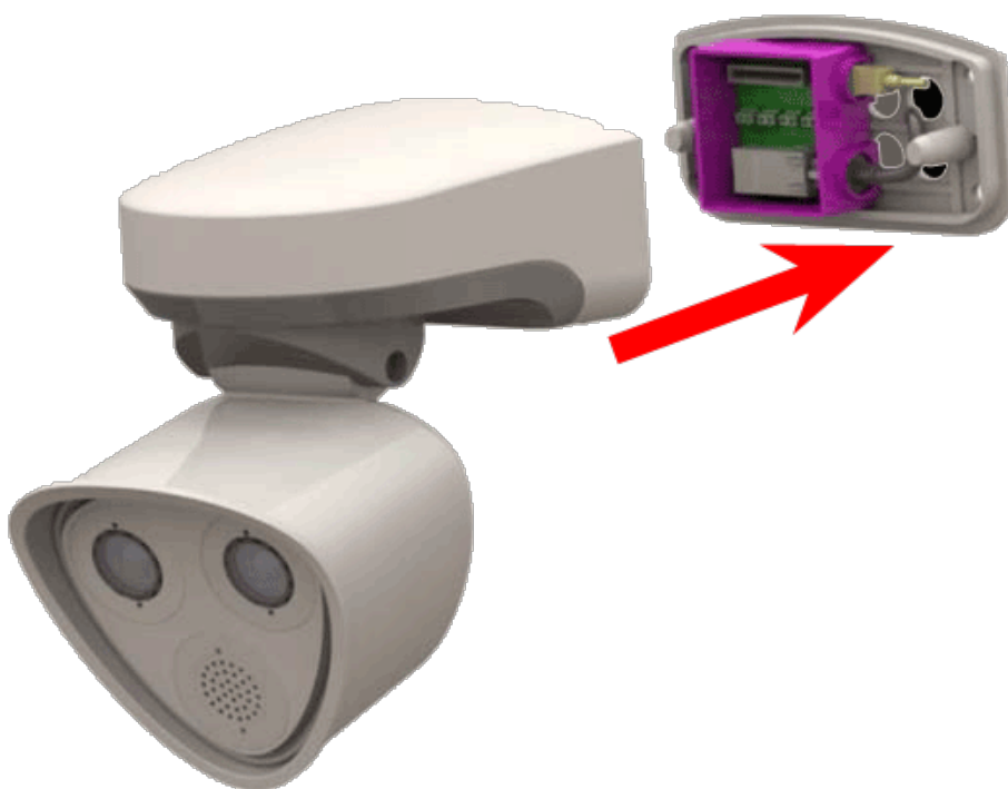
Fig. 70: Attach the camera on the mounting plate to complete the mounting of the camera
