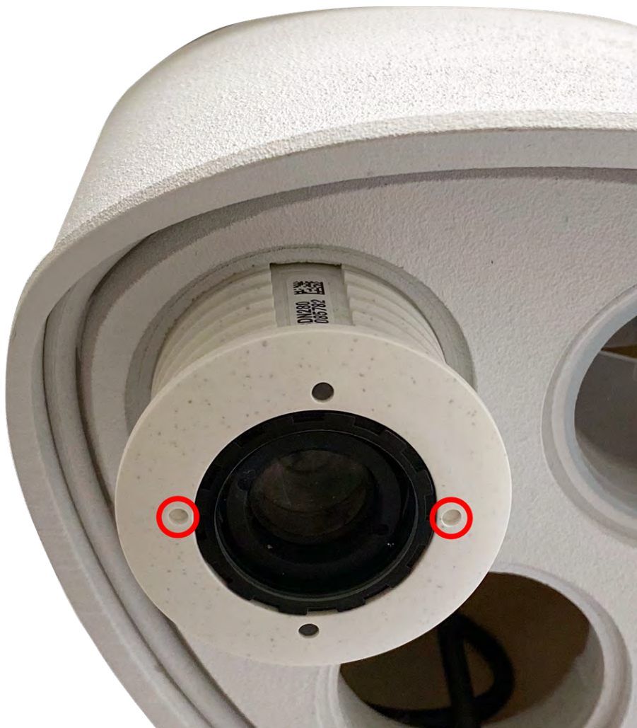
Fig. 12: Insert sensor module into module housing
