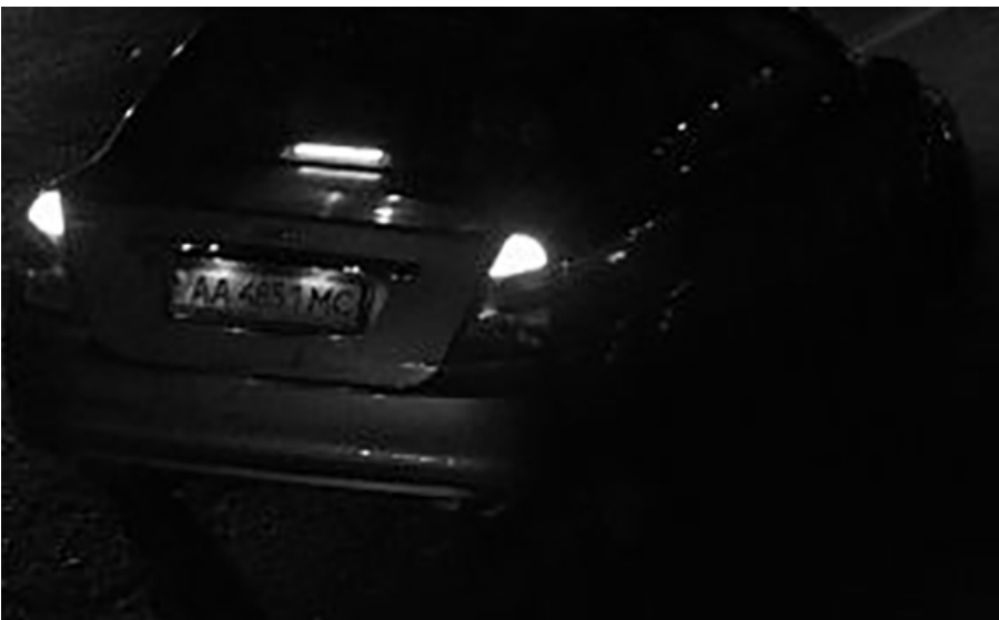
Fig. 15: Insufficient light to recognize license plate
