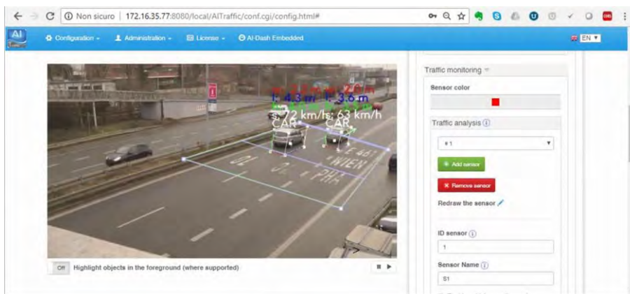
Fig. 75: AI-ROAD 3D: configuration
