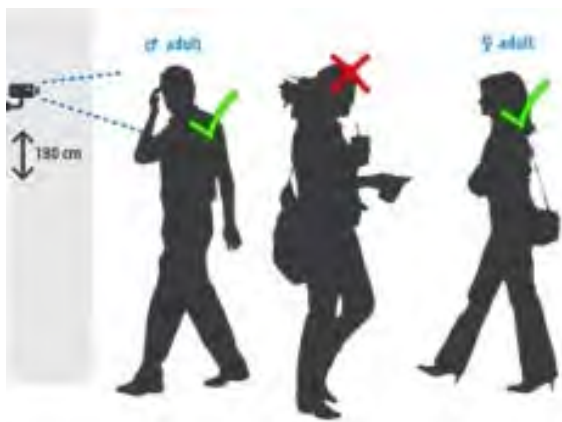
Fig. 59: AI-FACEDETECT-DEEP Camera positions
