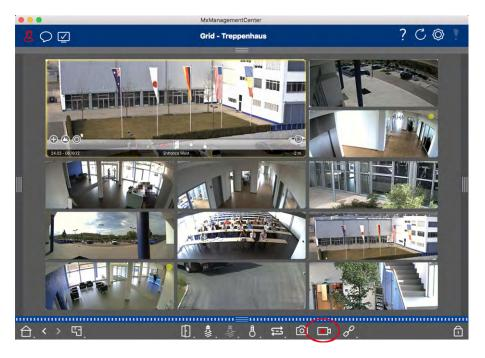
Fig. 21: Manually recording live images
