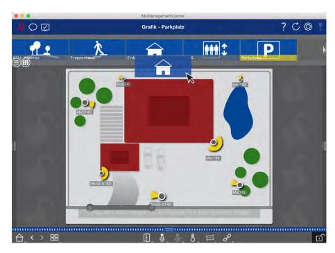
Fig. 104: Dragging additional camera group onto the background image
