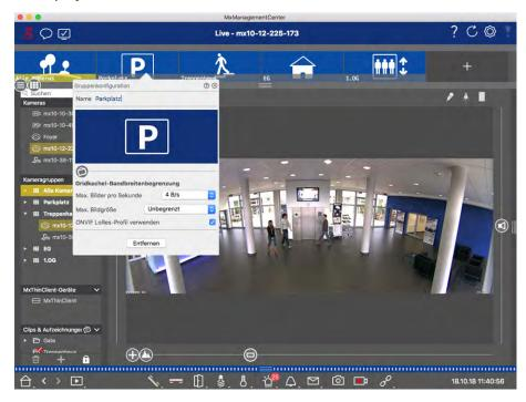
Fig. 107: Limiting the frame rate of live images
