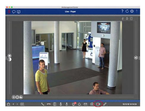
Fig. 6: Manually recording live images
