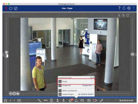
Fig. 110: Turn bell off completely
