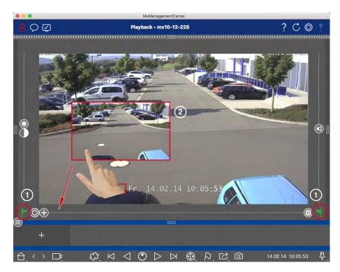
Fig. 87: Adding Clips for Exporting in the Playback View
