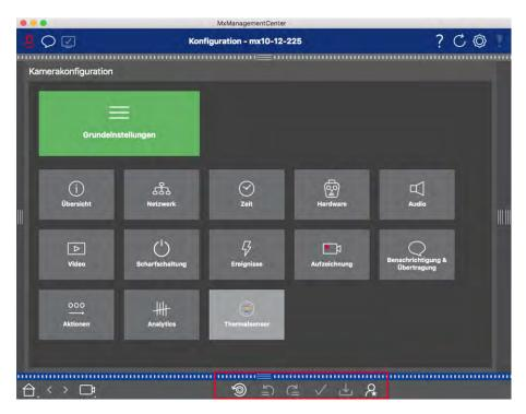
Fig. 40: Applying and saving changed settings
