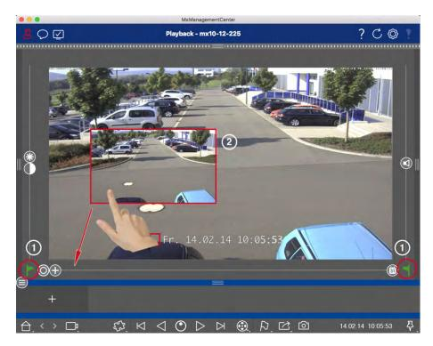
Fig. 17: Adding Clips for Exporting in the Playback View
