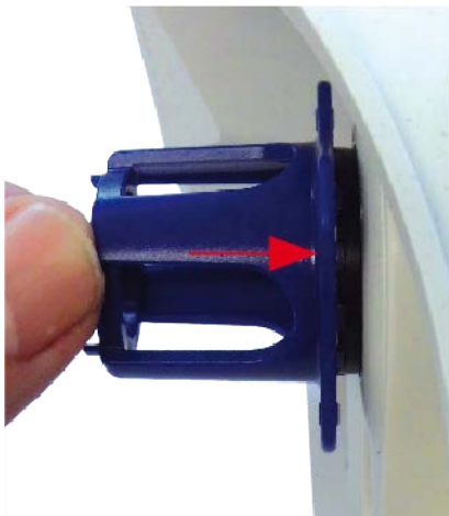
Fig. 87: Push hard to insert lens protection glass and turn to lock
