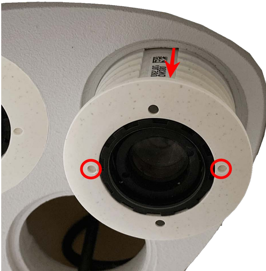
Fig. 23: Remove sensor module from the module housing
