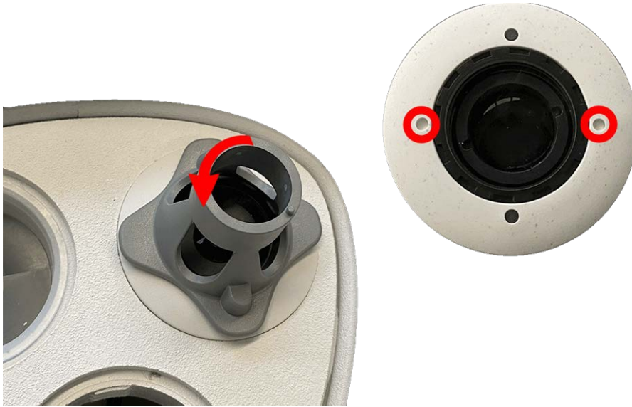
Fig. 22: Unlock the sensor module
