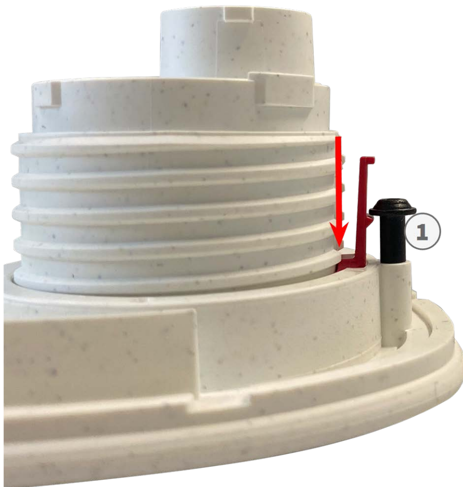
Fig. 17: Insert security clip all the way
