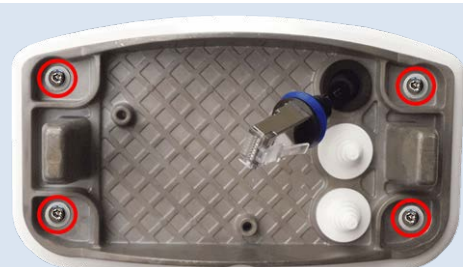
Fig. 50: Installed and ready for Connector Box RJ45
