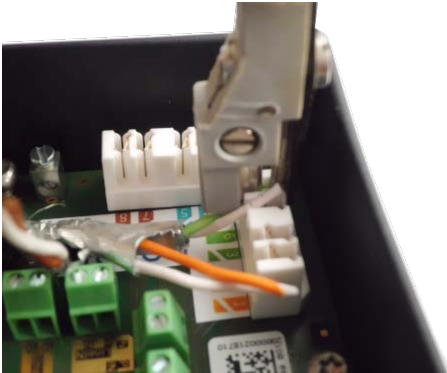
Fig. 63: Network wires connected using LSA+/Krone tool
