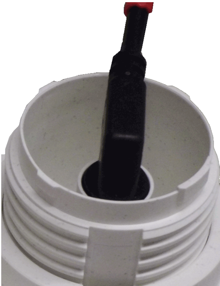
Fig. 10: Back of blind module with connector attached
