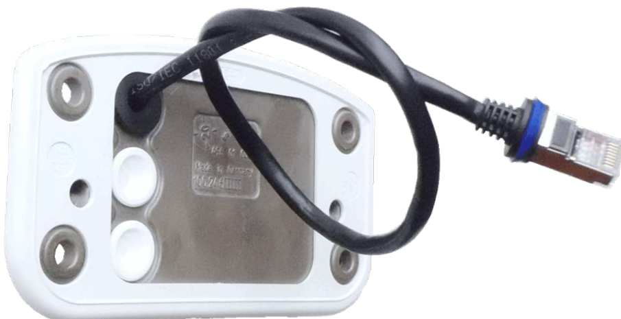
Fig. 32: Network connection of the M73
