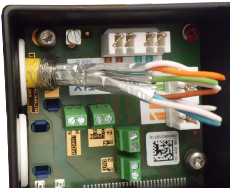
Fig. 60: Network cable inserted, plug properly seated
