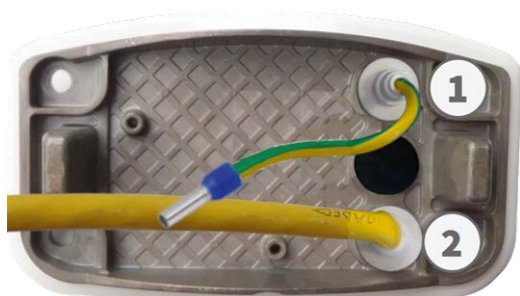
Fig. 35: Mounting plate with ground wire and network cable
