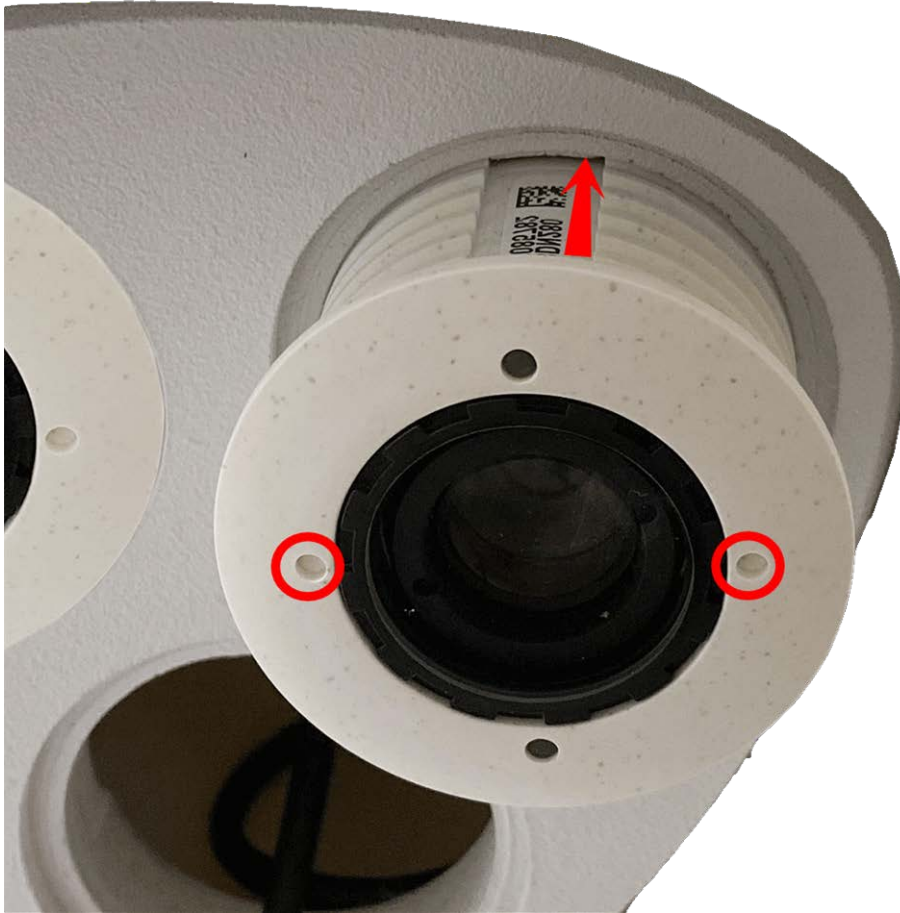
Fig. 25: Insert sensor module into Thermal front plate
