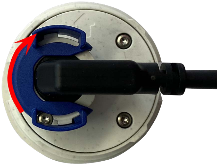
Fig. 11: Lock sensor module
