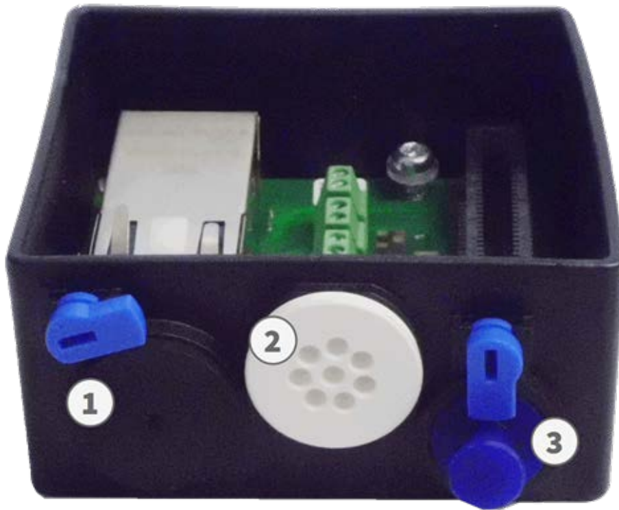
Fig. 53: Connector Box RJ45 with rubber plug black C.3 (1), rubber plug single-wire C.4 (2), USB plug (3) and two blue locks
