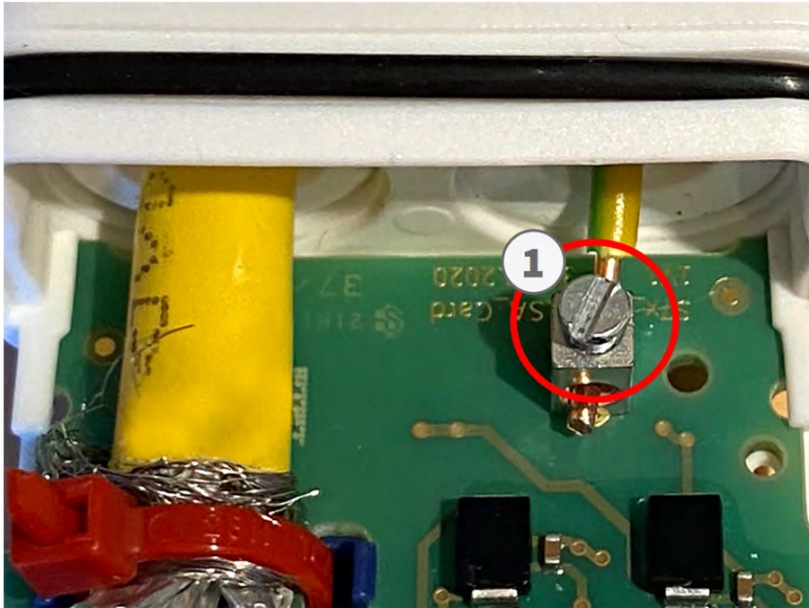
Fig. 29: Ground wire connected to terminal
