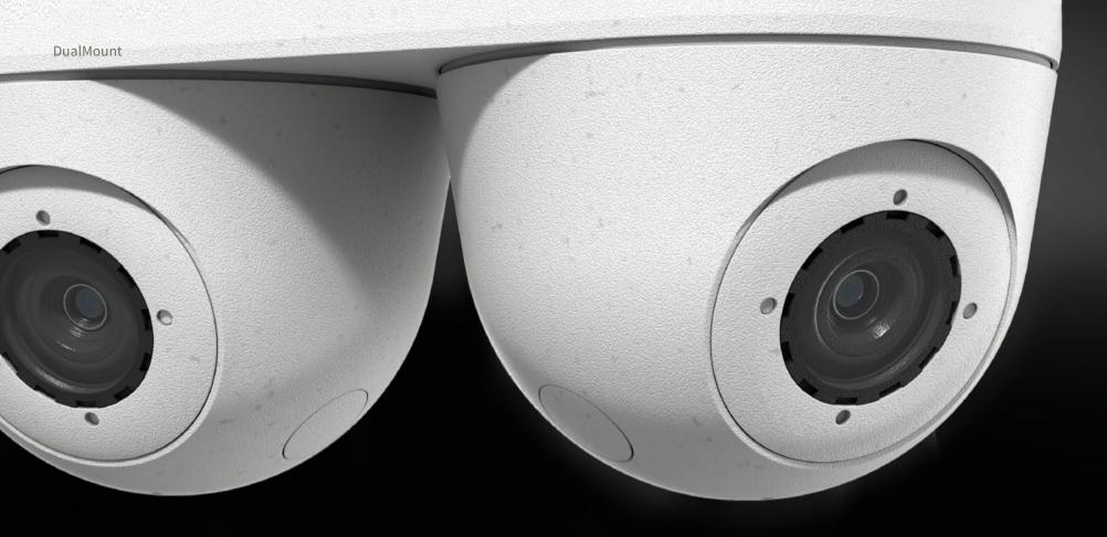
The S74 is positively chameleon-like: The eyes move completely independently of each other for the utmost **discretion and subtlety**. Fitted in the inconspicuous DualMount, two modules can be installed and oriented separately.
