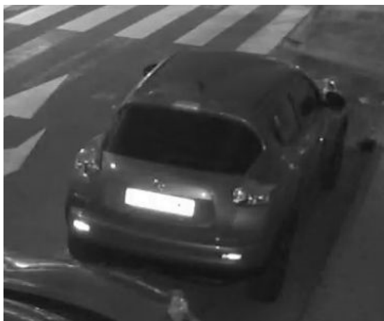
Fig. 14: Over exposed license plates due to too strong IR LED light
