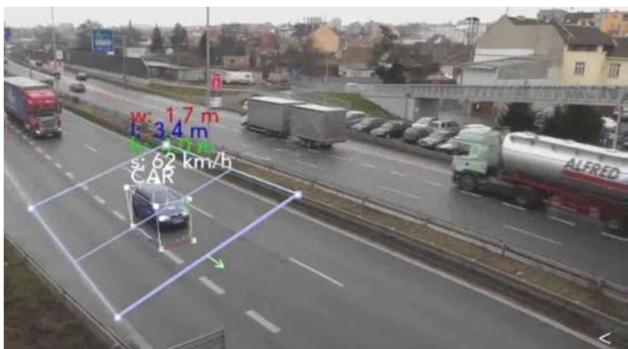
Fig. 92: AI-INCIDENT : configuration
