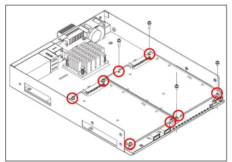
3. Mount the HDD onto the rack.
