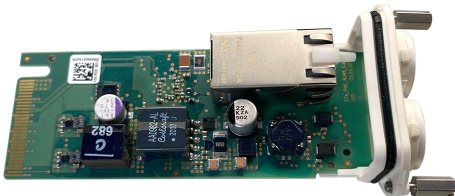
Fig. 17: Interface Board RJ45
