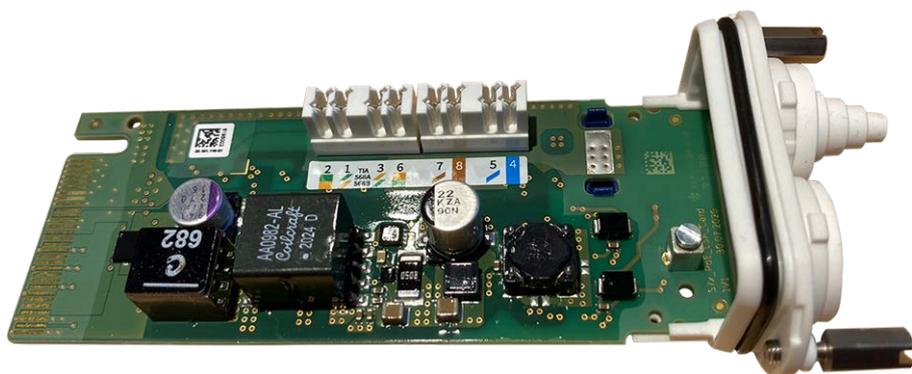
Fig. 20: Interface Board LSA
