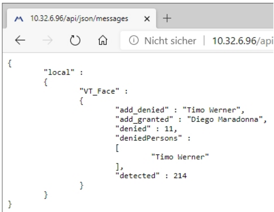
Fig. 18: Example: Meta data transmitted within an MxMessage of the Visage Technologies Face Recognition App
