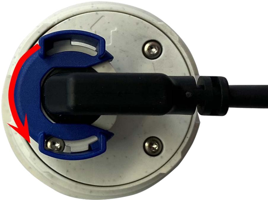
Fig. 20: Unlock sensor module cable
