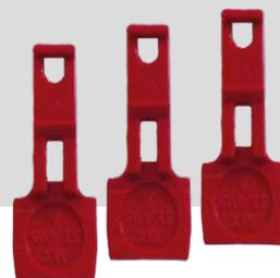
The security clips are protecting the sensor modules or the blind module in the front plate of the M73 against theft and unwanted rotation (e.g., due to vibration when mounted on a pole or in an automotive scenario). If they are installed, you need to remove them before you can remove the sensor modules.
