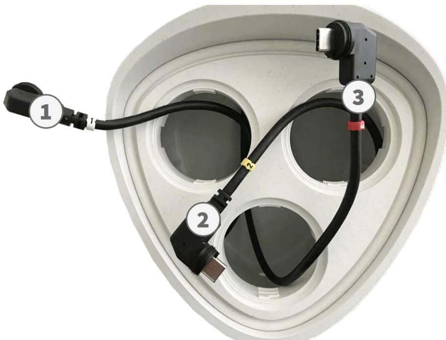
Fig. 8: Numbered sensor module cables
