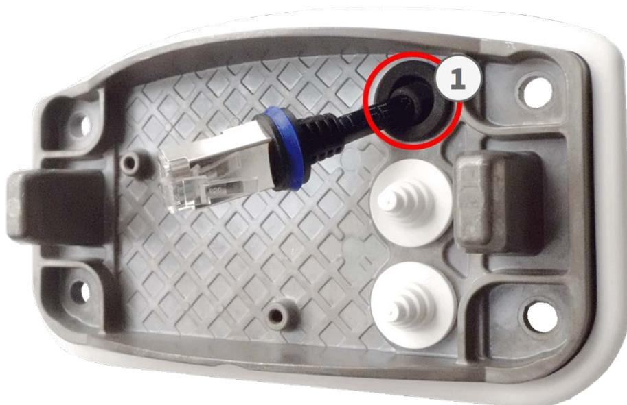
Fig. 47: Prepare the mounting plate
