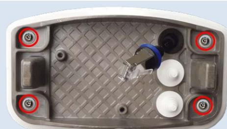
Fig. 36: Installed and ready for Connector Box RJ45
