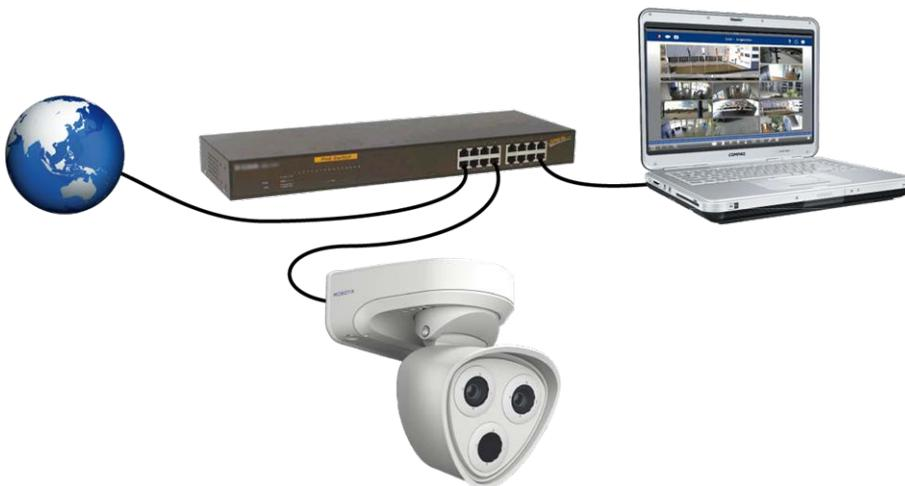
Fig. 52: Power supply using PoE switch according to PoE Plus (802.3at-2009)
