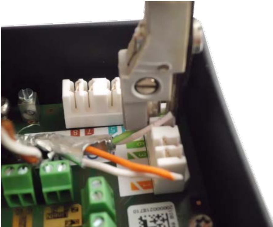
Fig. 63: Network wires connected using LSA+/Krone tool
