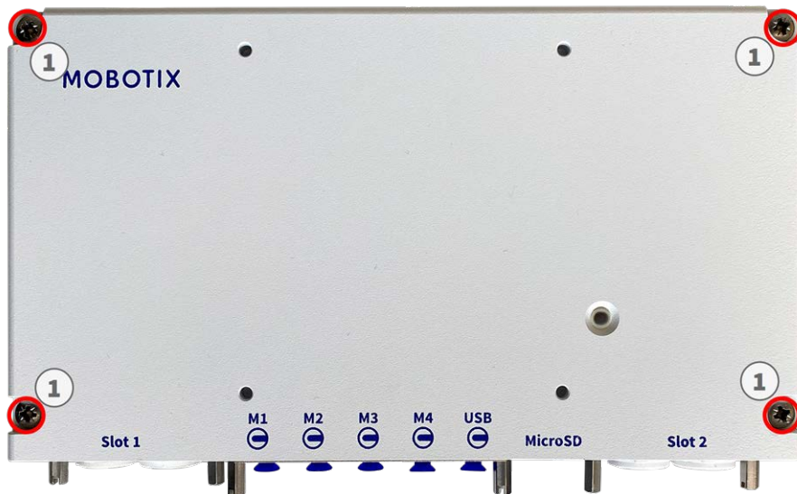
Fig. 31: Mounting plate installed on wall
