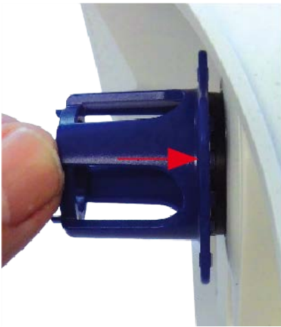
Fig. 48: Push hard to insert lens protection glass and turn to lock
