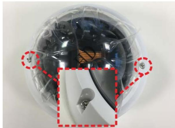
2. Open the back conduit entry block using a coin and place it to the side conduit entry.
