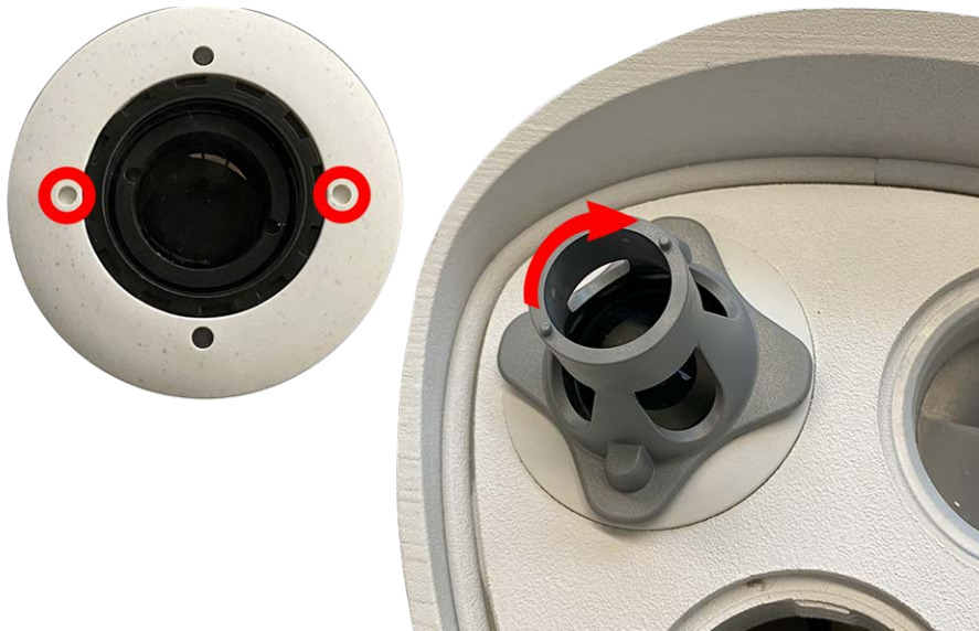
Fig. 13: Lock the sensor module
