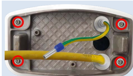
Fig. 37: Installed and ready for Connector Box LSA
