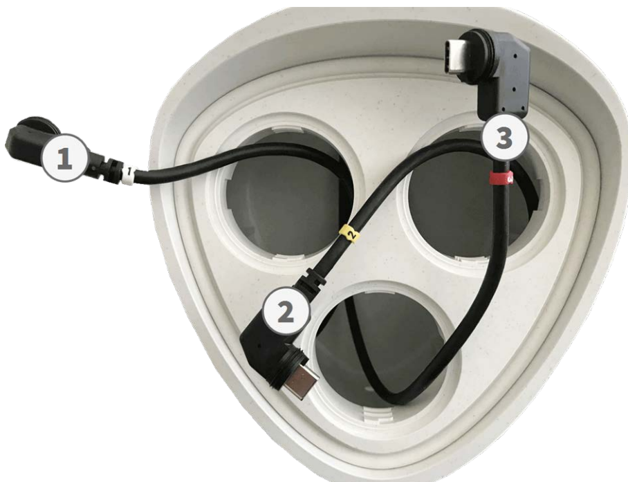
Fig. 8: Numbered sensor module cables
