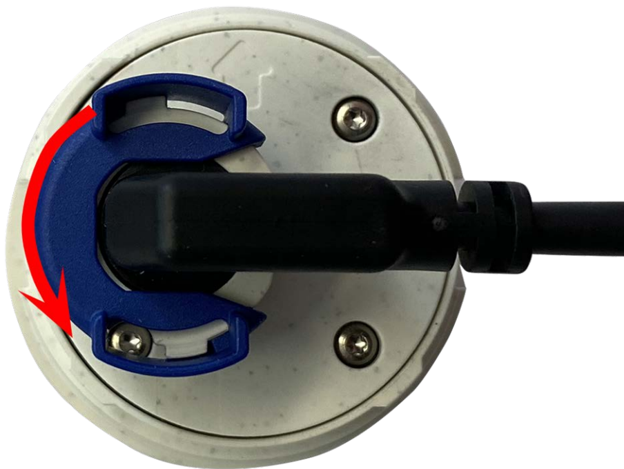
Fig. 20: Unlock sensor module cable
