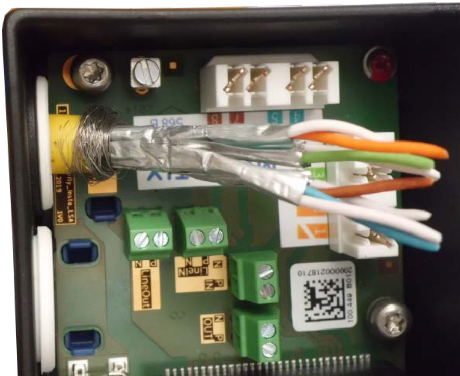
Fig. 60: Network cable inserted, plug properly seated
