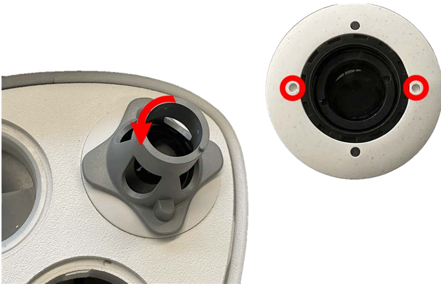
Fig. 22: Unlock the sensor module
