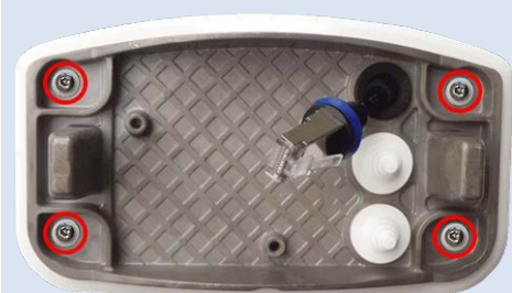
Fig. 50: Installed and ready for Connector Box RJ45
