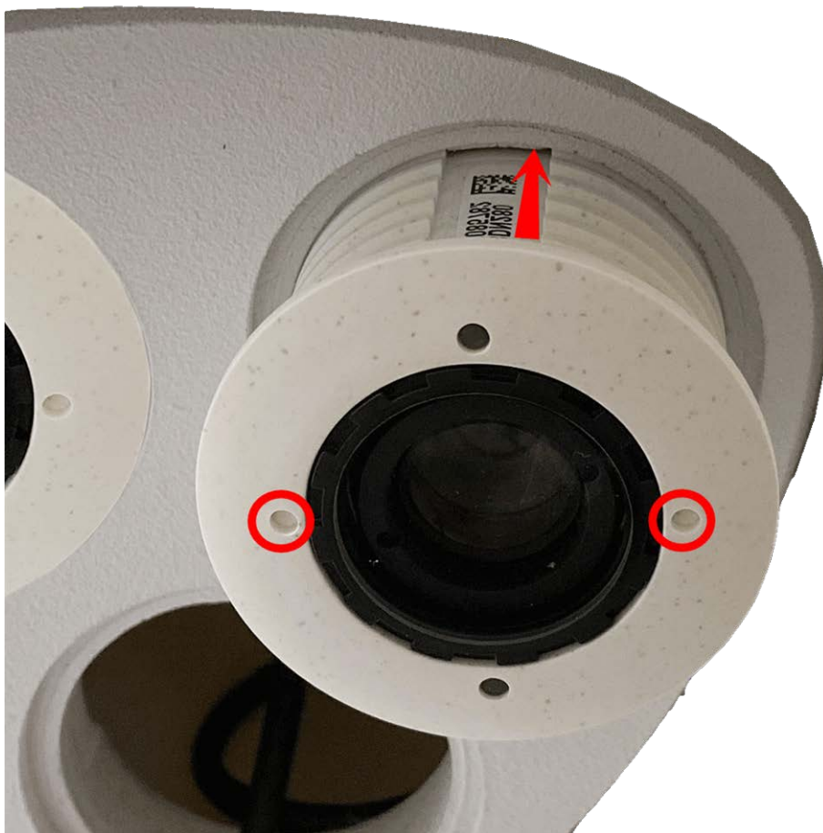
Fig. 25: Insert sensor module into Thermal front plate
