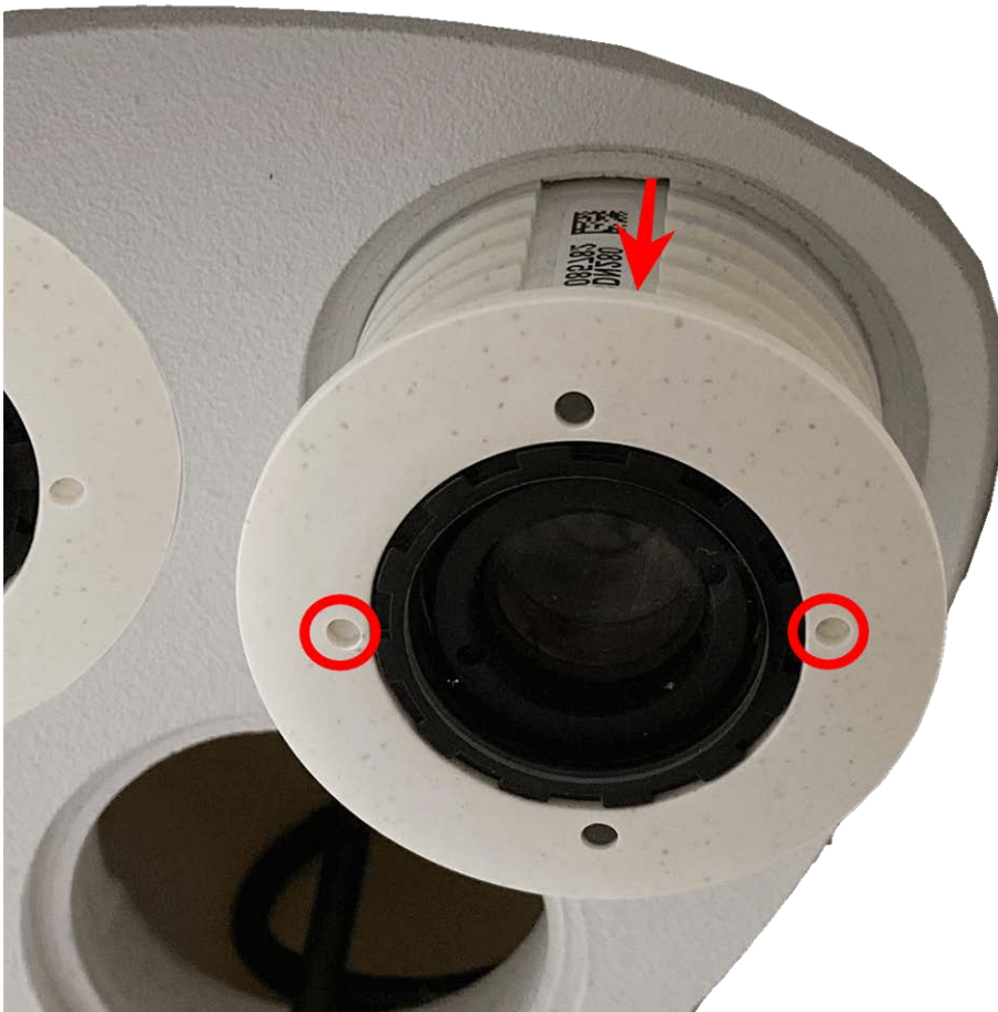
Fig. 23: Remove sensor module from the module housing
