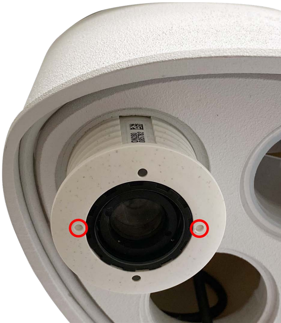
Fig. 12: Insert sensor module into module housing
