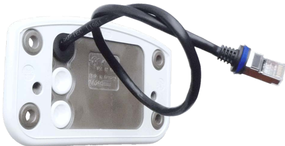
Fig. 32: Network connection of the M73
