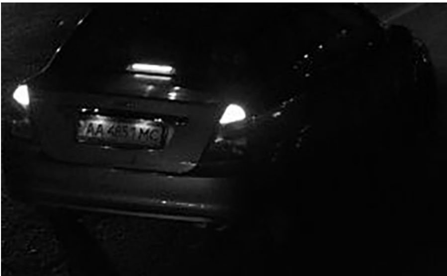
Fig. 15: Insufficient light to recognize license plate
