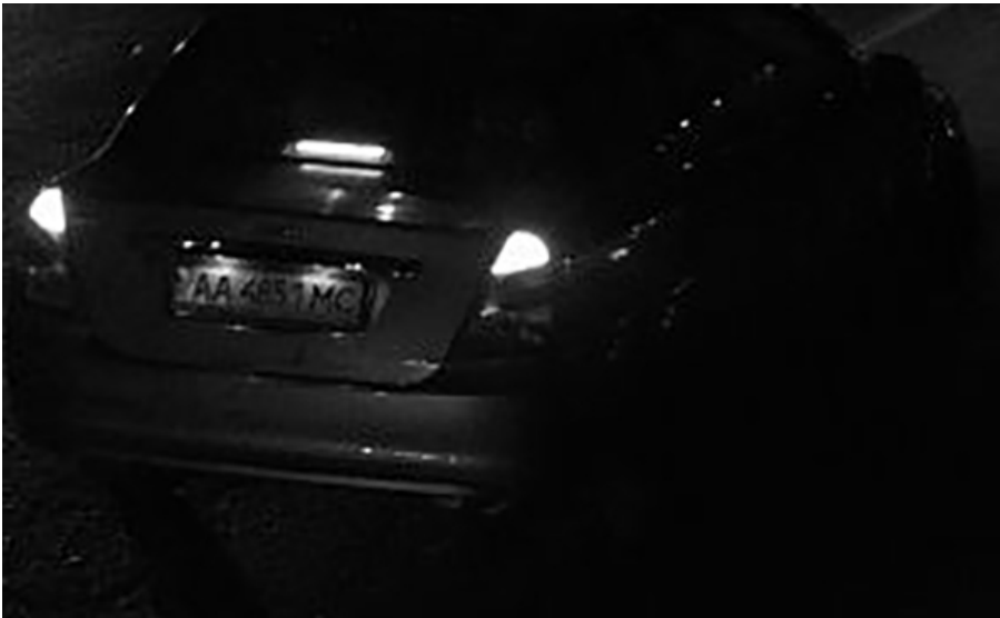
Fig. 15: Insufficient light to recognize license plate
