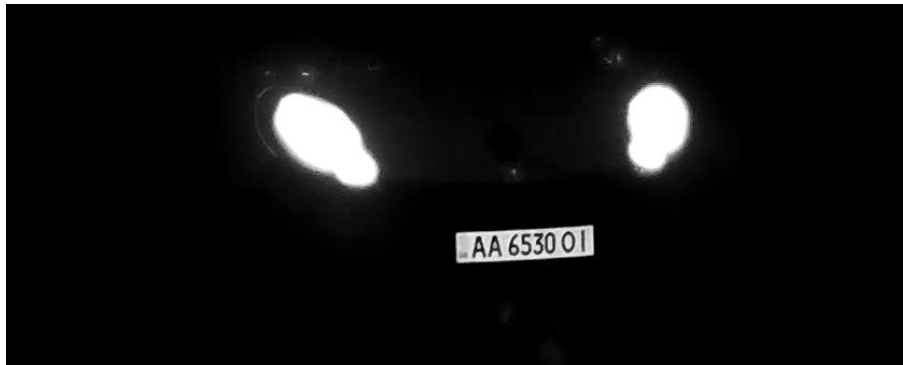
Easily readable license plate at night with infrared LED illumination
