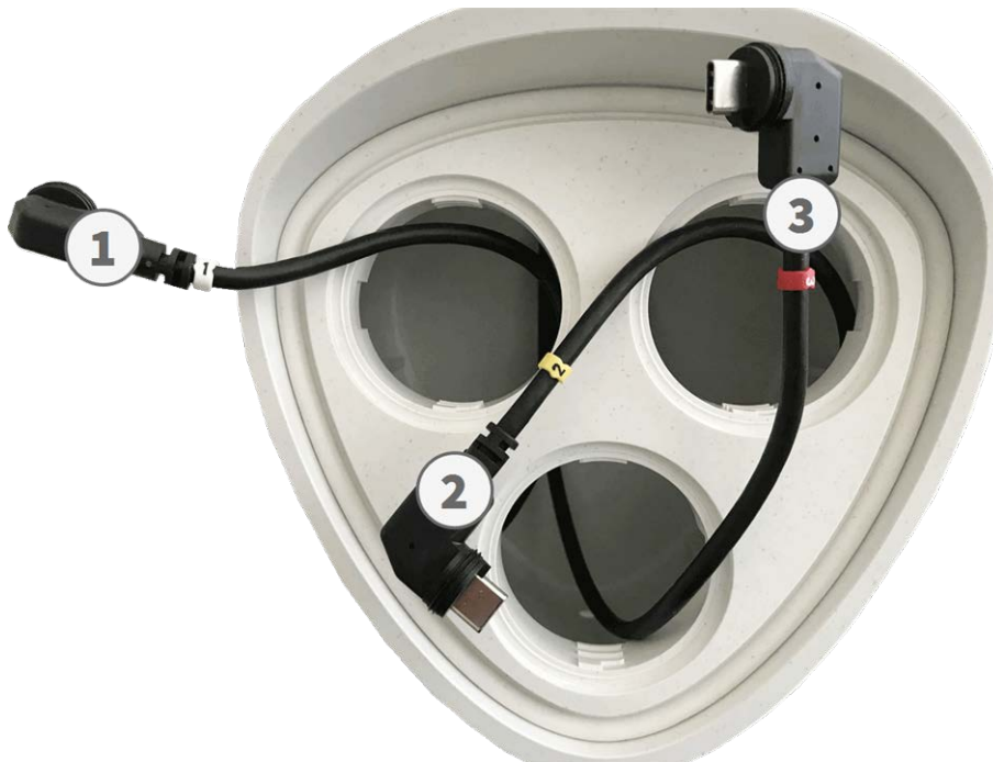
Fig. 8: Numbered sensor module cables
