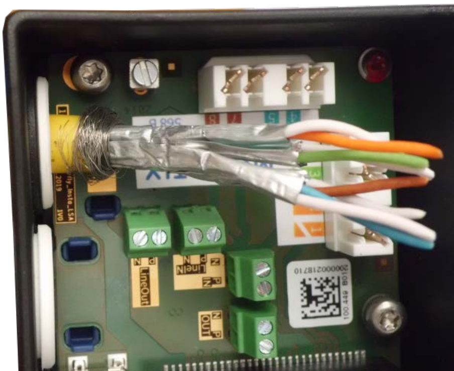
Fig. 60: Network cable inserted, plug properly seated
