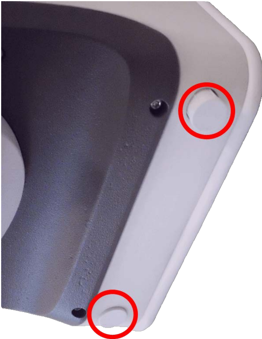
Fig. 71: Apply rubber plugs
