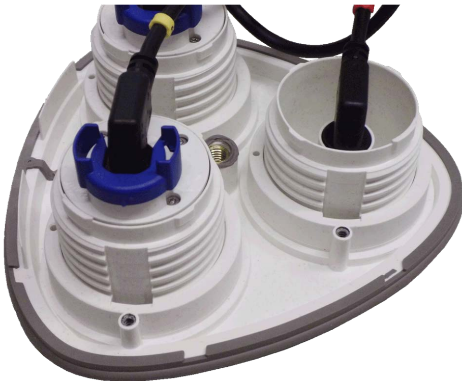
Fig. 15: Default front plate with sensor modules (back)
