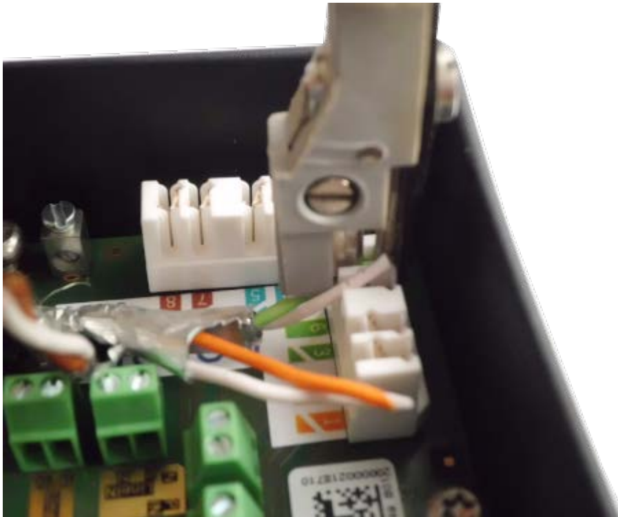
Fig. 63: Network wires connected using LSA+/Krone tool
