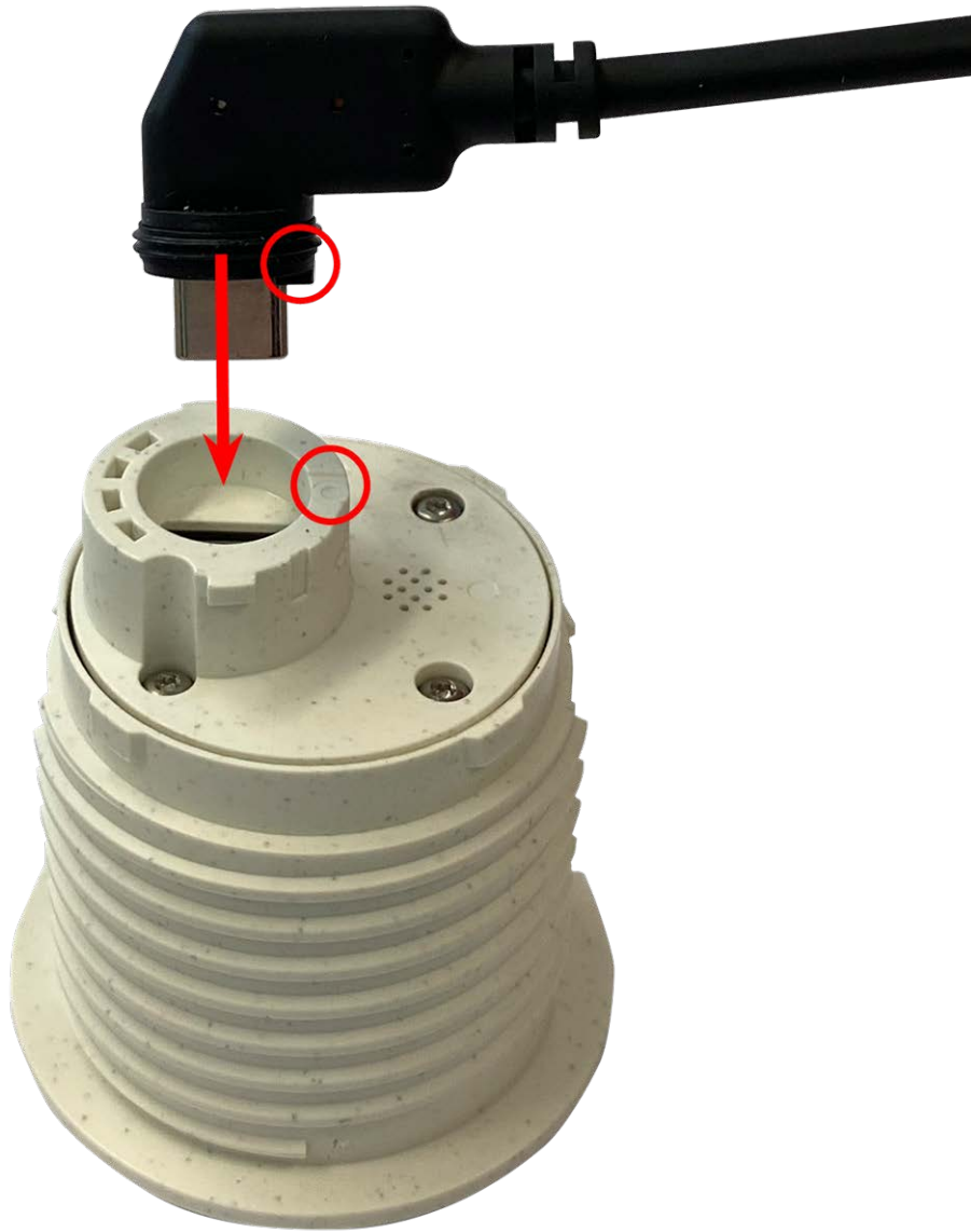
Fig. 9: Connect the sensor module cable
