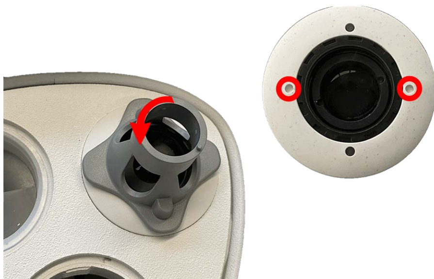
Fig. 22: Unlock the sensor module
