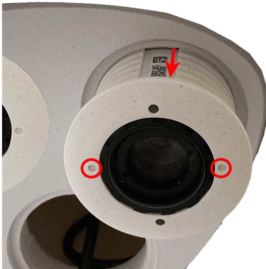
Fig. 23: Remove sensor module from the module housing
