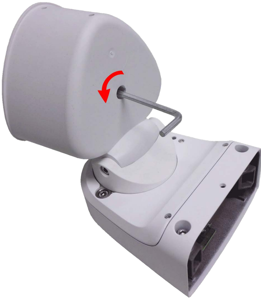
Fig. 14: Opening the module housing
