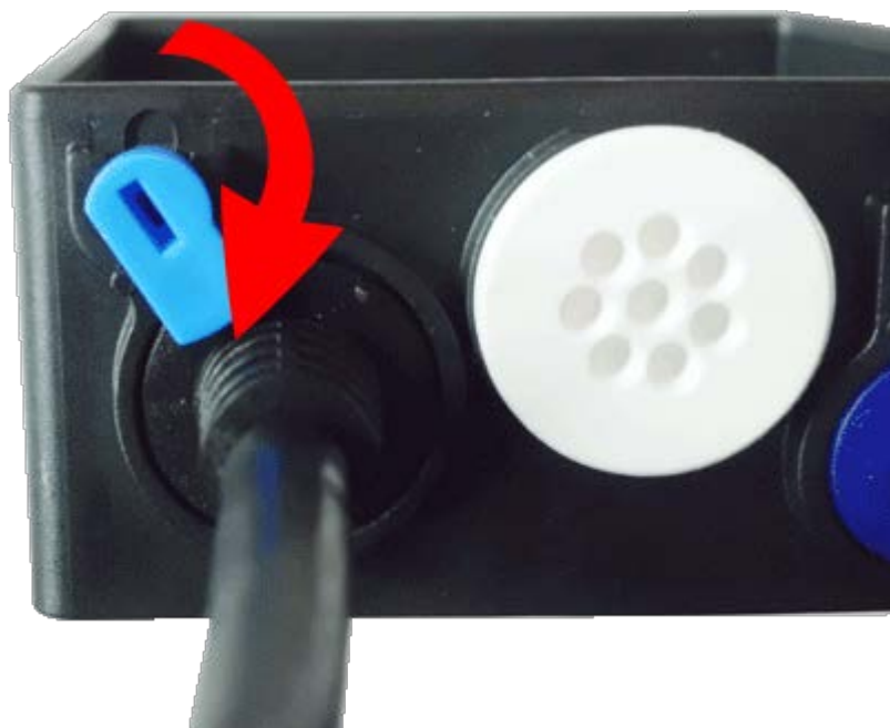
Fig. 54: Lock the network cable in the connector box
