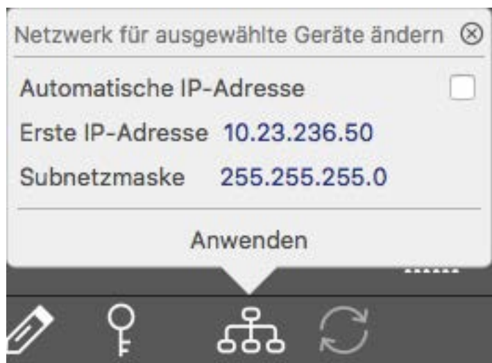
Fig. 80: Change network settings for selected devices
