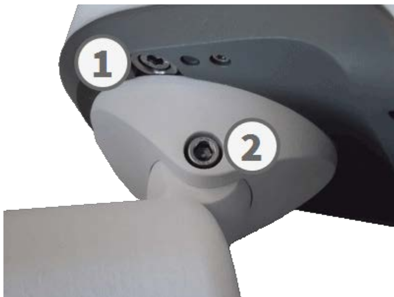
Fig. 72: Fastening the Camera
