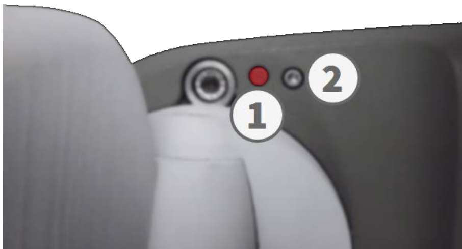
Fig. 74: View of the M73 from below with LED ① and screw with sealing ② that hides the key inside the camera body
