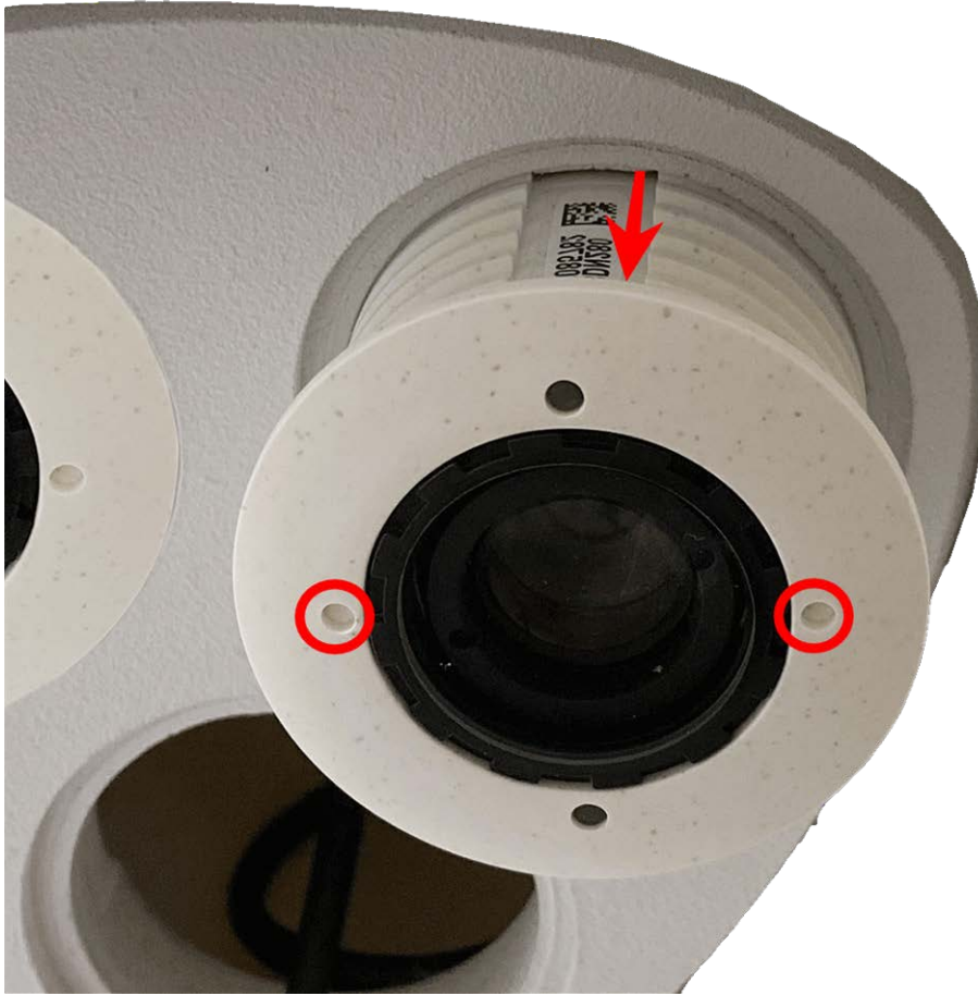
Fig. 23: Remove sensor module from the module housing
