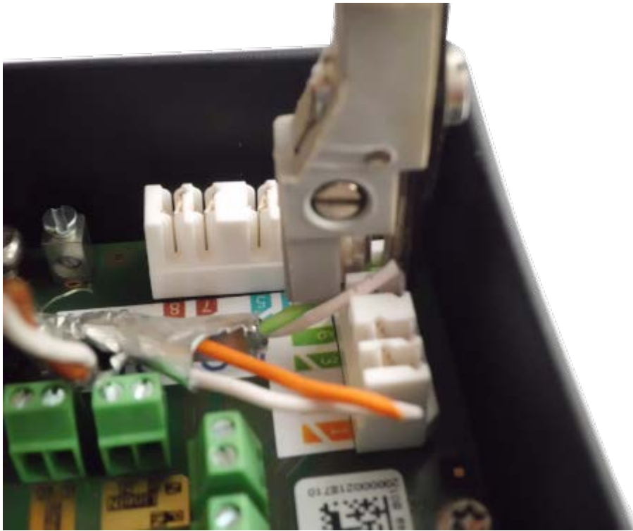
Fig. 63: Network wires connected using LSA+/Krone tool
