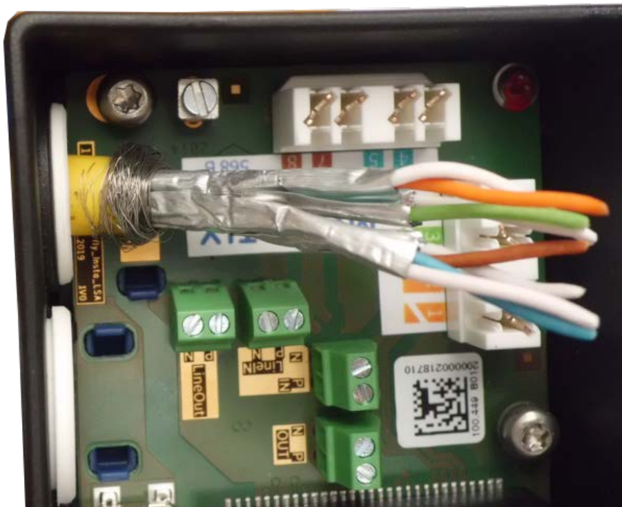
Fig. 60: Network cable inserted, plug properly seated
