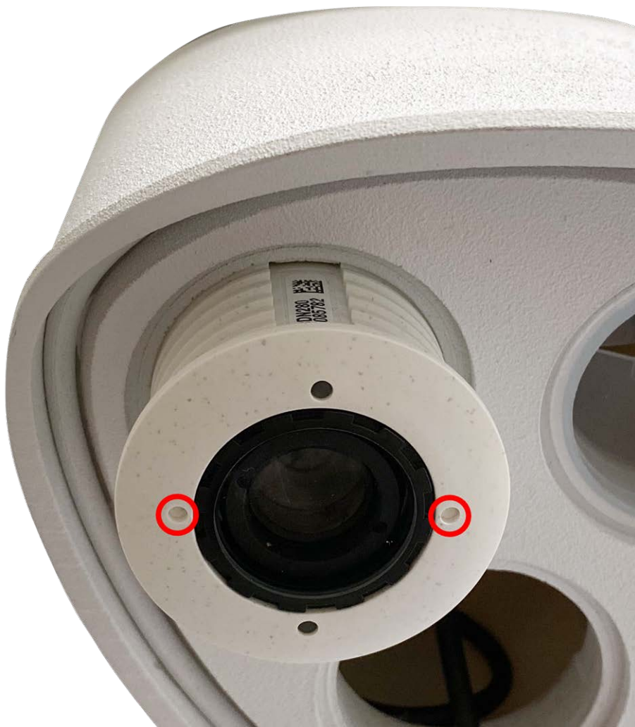
Fig. 22: Unlock the sensor module
