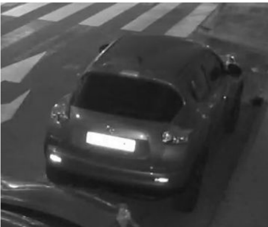
Fig. 14: Over exposed license plates due to too strong IR LED light
