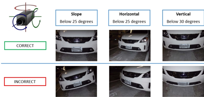
Fig. 11: Maximum rotation angle
