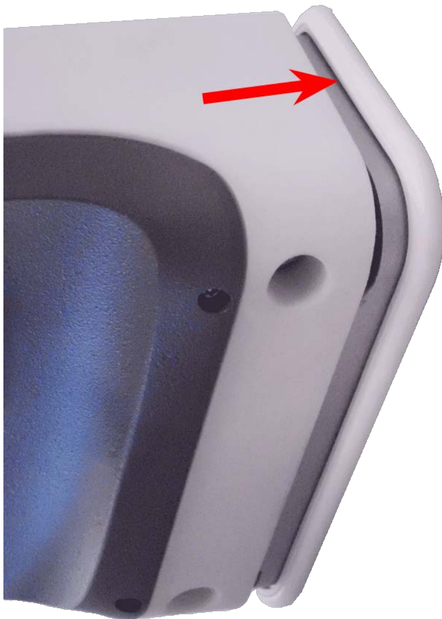
Fig. 69: Press camera onto mounting plate
